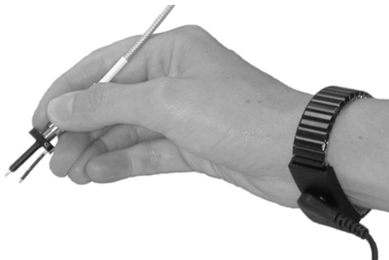
Figure 1. Correct method of holding the probe
